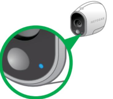
**Note:** The LED blinks amber if the sync is not successful. You must repeat the sync process.
