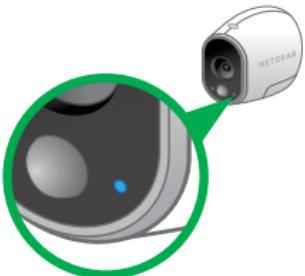
**Note:** The LED blinks amber if the sync is not successful. You must repeat the sync process.
